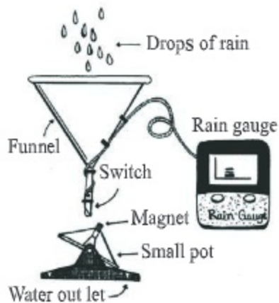
Figure : Rain gauge.
